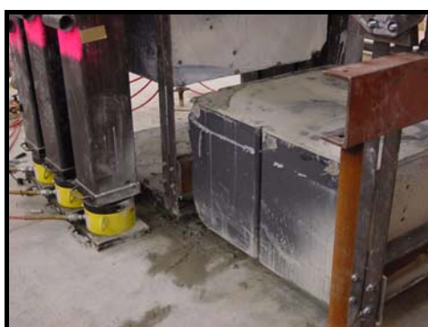
Concrete block removed from column
